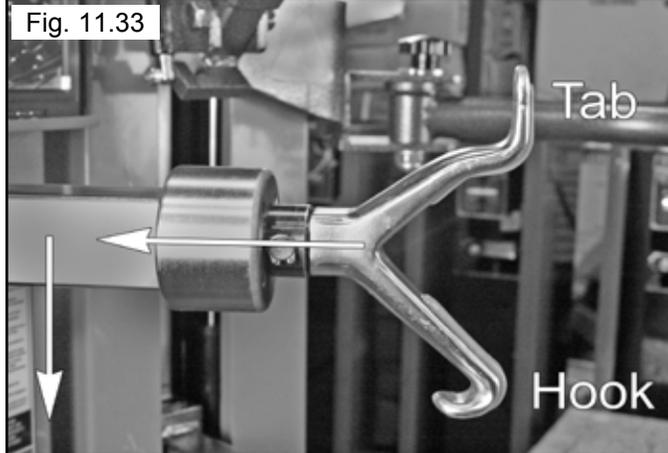
4. Position the Drop Center Tool as shown to bring the lower Bead up onto the Tire's Drop Center.
