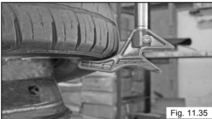
6. Push the Target Lock™ button and Hold, the Tool Head Tab will extend to the preset position 1/4" from the rims edge.
