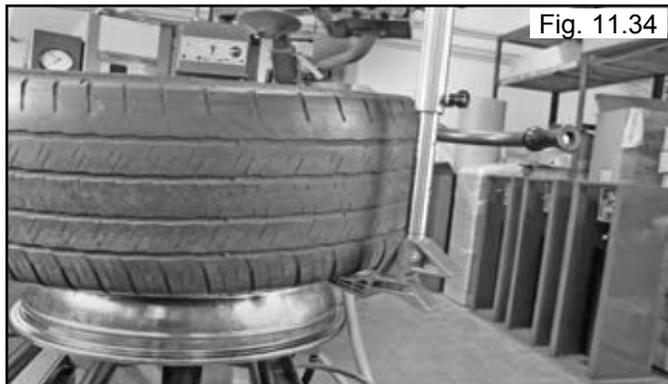
5. Raise Drop Center Tool until lower bead is in drop center. (See Fig. 11.35)
