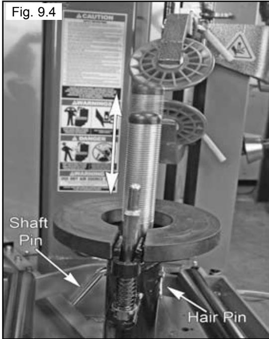
3. Align the holes and replace the Shaft pin and Hair Pin.
