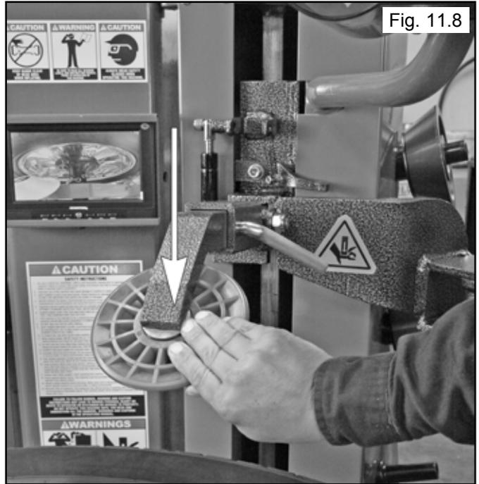
12. Lower the Upper Bead Breaker Roller to within about an inch of the tire Rim.
