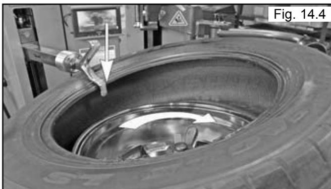
4. If necessary, for some stiff sidewall tires, use the Upper Bead Breaker Roller to help push the down on the tire, to Push bead below rim lip. (See Fig. 14.5)
