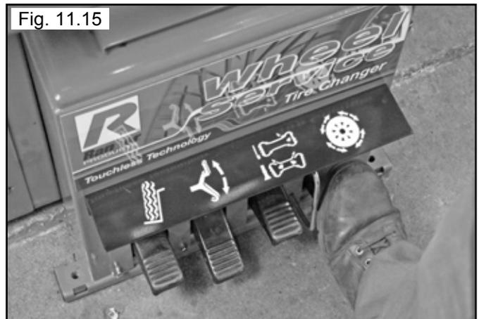
17. Pulse the Upper Bead Breaker switch down in small increments and the Lower Bead Breaker control up as the tire rotates to begin to break both the Upper and Lower Beads.
