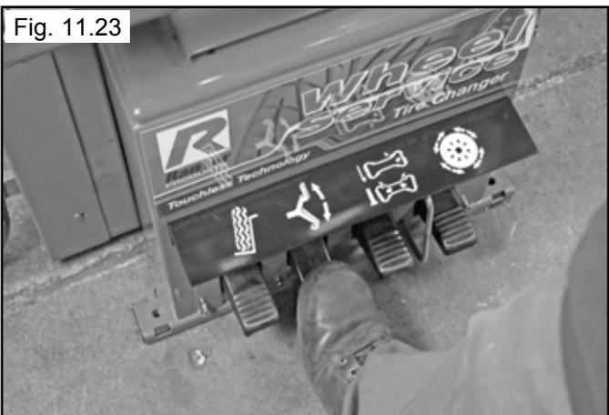
27. Using the Tool Head Control, lower the Tool Head down to just above the rim. (See Fig. 11.24)
