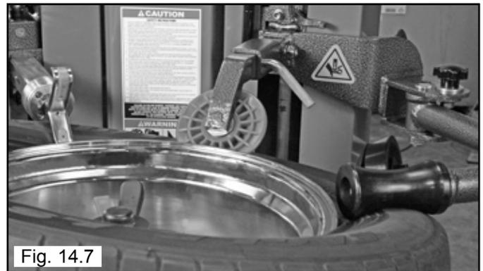
3. Lower the Drop Center Tool with the "mouth" side facing the rim and contact the tire just ahead of the Assist Arm Roller. (See Fig. 14.8)
