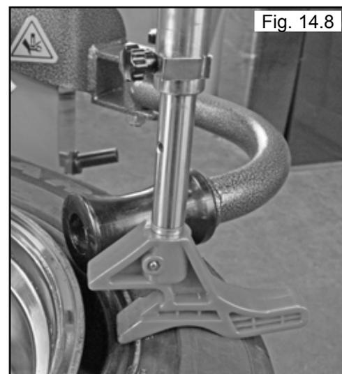
4. Lower the Drop Center Tool to Push the Upper Bead below the Rim's Drop Center. (See Fig. 14.9)
