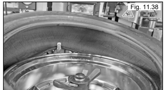
9. Keep the Lower Bead in the Drop center of the Rim.
