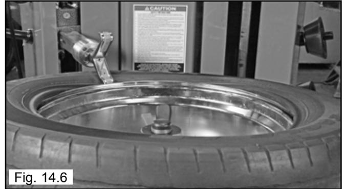
2. Lower The Upper Bead Breaker Roller and if needed, position the Assist Arm Roller to press the Upper Bead into the drop center of the Rim. (See Fig. 14.7)
