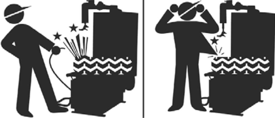
**STAND CLEAR WHILE INFLATING TIRE. TIRE OR WHEEL FAILURE UNDER PRESSURE MAY CAUSE SERIOUS INJURY OR DEATH.**
