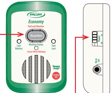
Slide the power switch to "OFF" to silence the monitor. Slide the switch to "ON" to reactivate the system.
