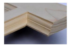
The construction will mimic that of cope and stick cabinet frame, only rotated 90 degrees making the stiles horizontal and the rails vertical. When routing the profiles, the top and bottom stiles will have just their inside faces routed. The edge rails will have the inside face routed in addition to a coping profile routed on the ends where they meet the
