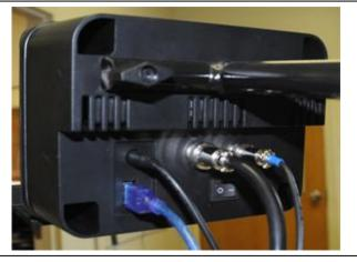
5. The control box has a shelf on it to hold your android device if you choose to set it up this way. Now you can connect your android device to the control box using the USB cable and micro adapter if needed. Your device should recognize you are connected to the lift when opening the MLCS PowerLift Pro App.
