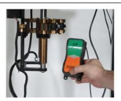
3. With the lift carriage in the lowest position insert the router motor into the carriage and lock it into place. You will want the top of the router motor just about flush with top of the carriage. Use the largest hex wrench to tighten the motor into position.
