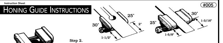
Use the wider jaws when sharpening plane iron. Position accordingly:  $25^{\circ}$  angle — project 2" from edge of jaws  $30^{\circ}$  angle — project  $1\frac{1}{2}$ " from edge of jaws
