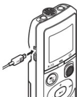
This voice recorder can also be connected to a PC, and used as mass USB storage. This is convenient for transferring large files such as image data between computers.
