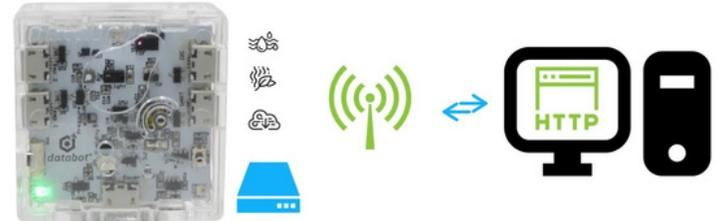
When you connect to databot™'s **local network** in Server mode you can configure databot™ to store data in **internal memory** for later download or access other services such as the **Environmental dashboard**.
