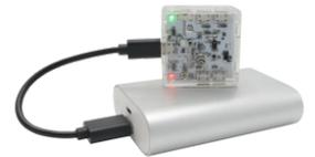
The charging port is the one oriented to the back of the case – you will see a single, micro-USB port in the center of the board to the right of the on/off switch.
