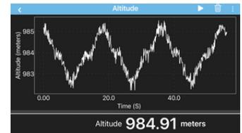
in determining your relative changes in altitude. For example, the Vizeey™ screen capture above shows walking up and down a set of stairs and the results were accurate to within less than two inches.
