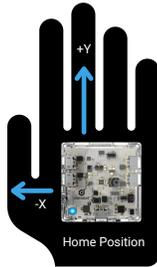
Start by shaking databot™ on each axis so that you get each axis to display an equal range of -20 to +20 m/s<sup>2</sup>.
