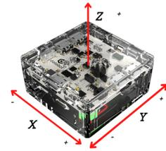
Meet the Accelerometer
