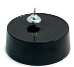
Give this top a spin and watch it move for hours without stopping. What's the secret? The top contains a small magnet. When this magnet moves past the center of its base, the top's spinning magnetic field induces a current in a coil, which closes a switch, allowing a battery to momentarily energize a small electromagnet. The top increases its rate of spin and moves away from the center of the base.
