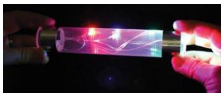
Safely demonstrate open and closed series circuits without any danger of electric shocks! When the tube is ‘turned on,’ the red, green, and blue lights light up and it makes a funny buzzing sound. Turning the tube on is the fun part - just touch the metal ends with both hands. Your body forms the conducting material that bridges the gap between the two metal strips and closes the circuit!
