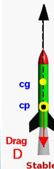
A stable rocket has its center of pressure (cp) behind the center of gravity (cg).
