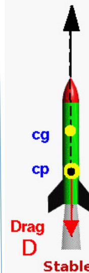
A stable rocket has its center of pressure (cp) behind the center of gravity (cg).
