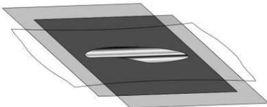
3. Place a piece of polyethylene between two crossed polarizing filters. Then stretch the polyethylene by pulling it. Examine the stretched polyethylene sheet between the filters.
