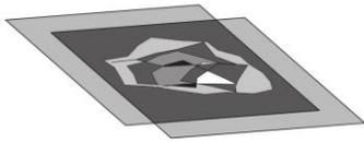
1. Place a piece of mica between two crossed polarizing filters. Each color represents a different thickness of the mica. Try rotating one polarizing filter. Try rotating the mica.
