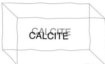
5. If you look at the words on a printed page through a crystal of calcite, you will see double. These natural, nearly transparent crystals exhibit the property of “birefringence,” i.e. they break light into two distinct polarized beams. By rotating a polarizing filter over the crystal, it is possible to view one image at a time. This phenomenon can be displayed using an overhead projector.
