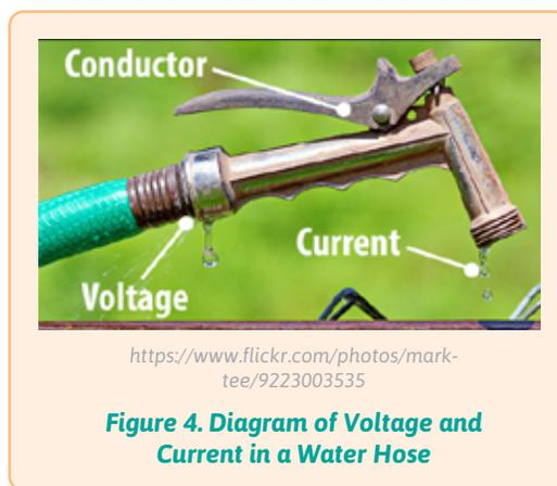
Figure 4. Diagram of Voltage and Current in a Water Hose
