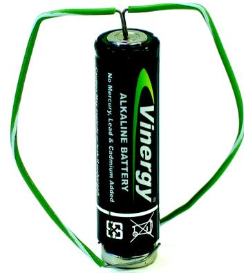
Fold the wire in half to find the exact center point. Strip the center of the wire to create a pivot point. Also strip about 1 cm at the end of each “arm” (Alternatively, you could strip the entire wire.)
