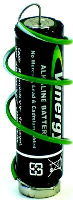
Wrap the wire tightly around the battery making a coil of wire. To make a pivot point, bend one of the stripped ends to make the tip of the wire point through the center of the coil.
