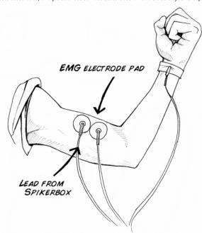
2. Hook up the Muscle SpikerBox leads (the 2 red alligator clips) to the two surface electrodes on your bicep.
