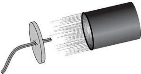
These amazing piezoelectric devices generate a few thousand volt sparks at the touch of a button. No batteries required. The discharge is created when a small hammer inside the device strikes a quartz crystal. It can be used as a safety lesson to demonstrate the flammability of alcohol or perfume. Igniting two drops of alcohol in a film canister will cause the canister to fly more than 20 feet into the air!
