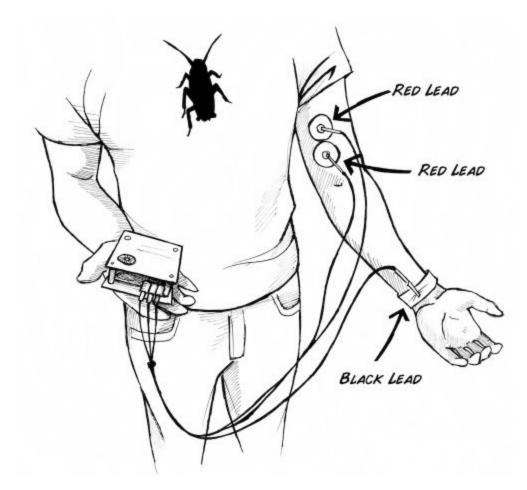
3. Place the reference electrode (Black) anywhere on the body. In the figure above we show it attached to a metal bracelet near the wrist. You can also use another EMG electrode placed anywhere on your body, or if you have any metal rings on your fingers, you can clip the reference electrode to your ring. Marriage has many advantages! You can also simply hold the reference electrode in your hand.
