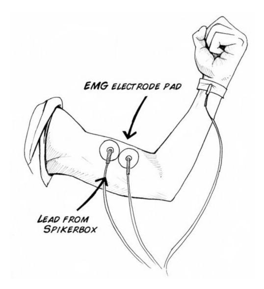
2. Hook up the Muscle SpikerBox leads (the 2 red alligator clips) to the two surface electrodes on your bicep.
