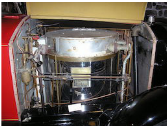
Steam engine in a 1924 Stanley Steamer
