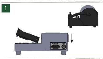
Attach the MaxVac Roll Holder & Cutter to your MaxVac.
