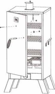
Install handle as pictured using the included washer and nut. Thermometer will come pre-assembled on the door.
