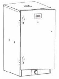
Door is easily removed by simply lifting straight up off the hinges.
