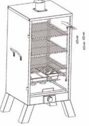
"S" hooks can be installed on the "U" brackets and used for hanging sausage casings.
