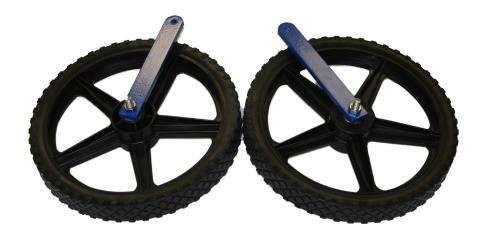
Apply a drop of Loctite 242 or equivalent threadlocker to each of the nuts prior to installation. Screw the nuts in place and tighten. After tightening, ensure the wheels spin freely with little to no noticeable drag. If there is noticeable drag, back the nut off by 1/8 to 1/4 turn until the wheel spins freely.
