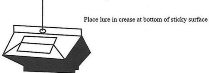
3. Hang the trap by placing a twist-tie hanger through the hole in the top of the trap and hang in an appropriate location. Inspect the traps regularly and remove insects and debris. Replace diamond trap as neccessary when sticky surface becomes covered with debris, dust or insect scales.
