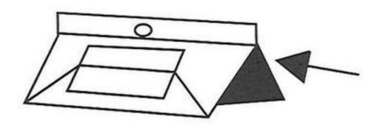
Grasp here and pull down to pull trap into place
